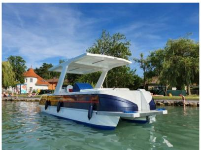
Boat length: 26 feet Ownership: company Built: 2024 Maximum length: 8.5 m Maximum width: 2,48 m Max. number of persons carried: 12 Engine: Siemens léghűtés 12kW Weight (kg): 2200 kg
